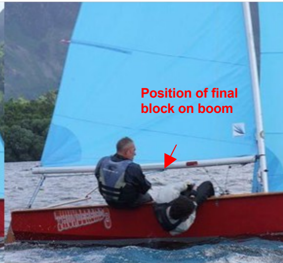
Figures 2a and 2b: Peter Lawson and Gareth Balfour in action at Inlands at Bassenthwaite in 2008. Note positions of rope loop and final block. – Photograph Bassenthwaite SC.
